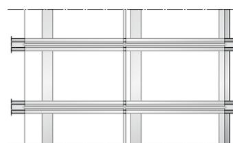
Horizontal rails (fixed on vertical profiles)
